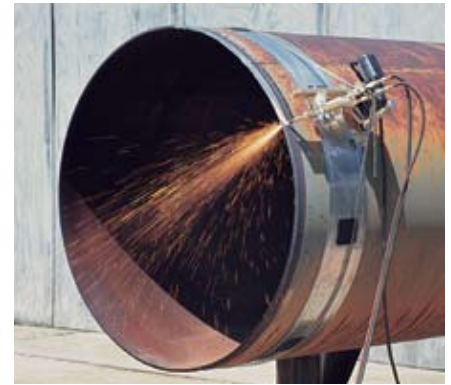
Band Style Cutting 48" Pipe
