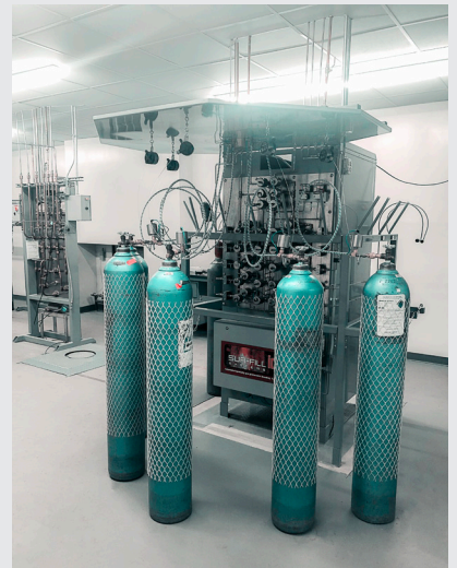
© Weldcoa | The new manifolded fill system automatically vents, vacuums and fills tanks
